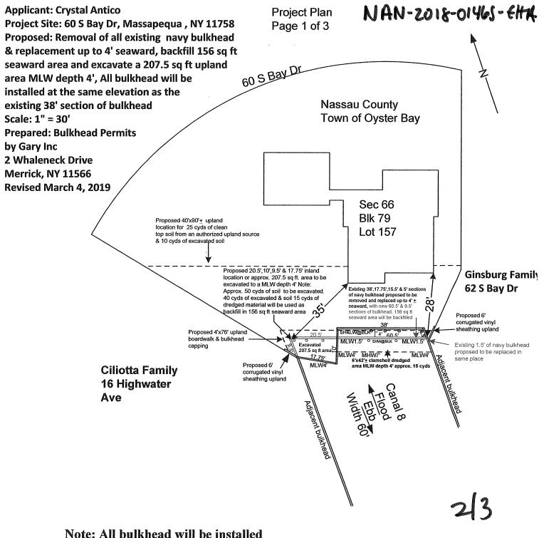
at same elevation as existing 38' section of bulkhead
